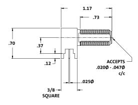
Lengthened D-cut Right Angle PCB Mount
