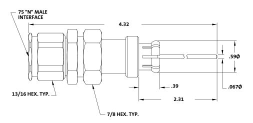
Precision Lab Grade N Male - Quick Disconnect KS Port Adapter
