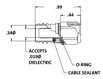
Universal Series 59/6 Crimp Connector & Weathergrade Universal Series 59/6 Crimp Connector
