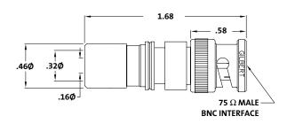
UltraSeal BNC for Headend Cable Compression Connector
