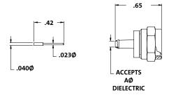
Conformable Coax Solder Connector
