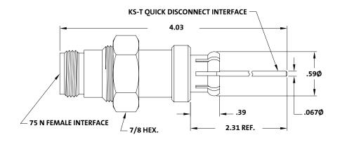
Precision Lab Grade N Female - Quick Disconnect KS Port Adapter
