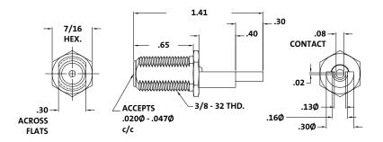
RG-179B/U Direct c/c Solder Coax Connector
