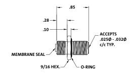
2 GHz Moisture Sealed Panel Mount Splice
