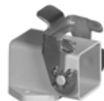
C146 10F 003 0044 Surface Mount Base Angled, Open 1 Lever, Plastic W 41 L 40 D 26
