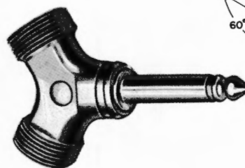
⊕ Part No. 330M Connects two cables with standard female microphone connectors (such as Switchcraft No. 2501M) in parallel to standard .25-in. (6.35 mm) phone plug output.
