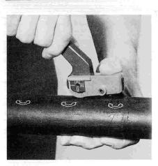
**6.** For longitudinal cutting of uncut cables, use eccentric position IIII. The cable sheath is cut by holding the blade against the cable sheath and pressing down the hand lever.
