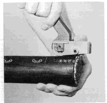
**4.** The eccentric unit has been adjusted correctly, if the plate of the cutter is parallel with the cable, while the blade is inserted under the cable sheath.
