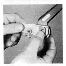
**3.** Adjust position I, II, III, or IIII according to the wall thickness of the cable sheath by turning the eccentric unit with thumb and forefinger.
