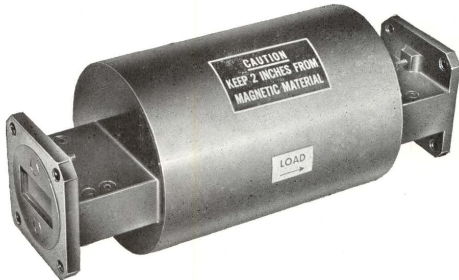
This ferrite isolator has been designed especially for test equipment applications and has a very high performance over an extremely broad frequency range. Covering all of the commonly used frequencies in X-band with no adjustments whatever, this single unit takes the place of the usual buffer attenuator between RF oscillator and waveguide bench.
