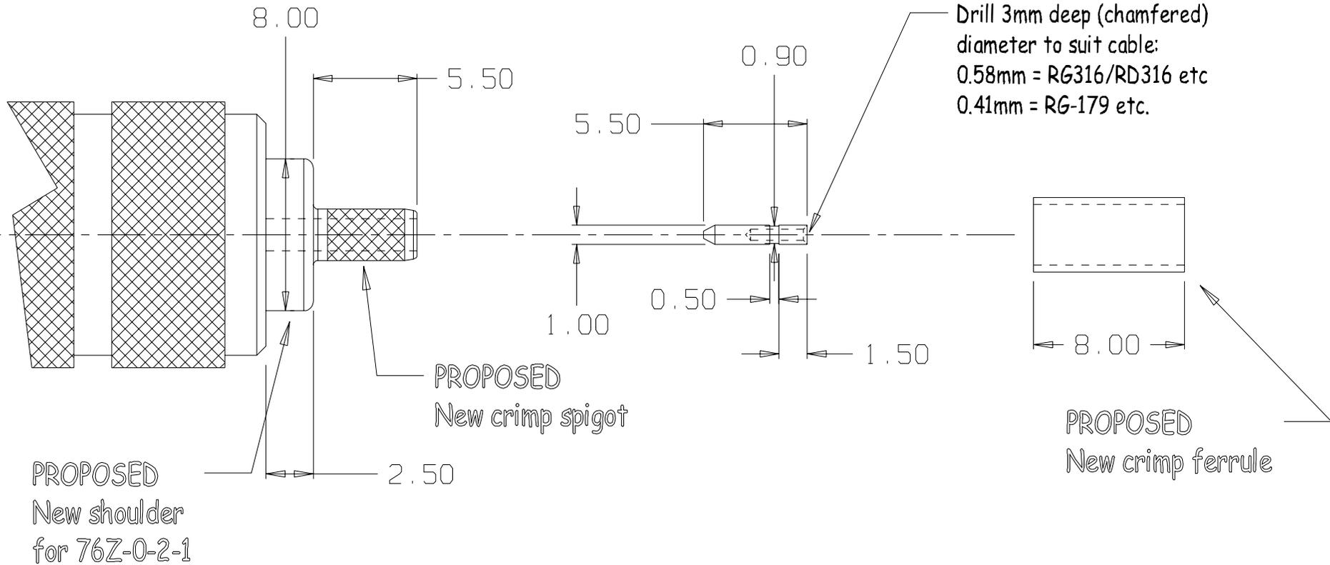
Note: This pin provides for the use of contact-registration/location finger such as is included in Suhner crimp die 76Z-0-2-1
