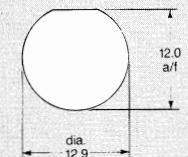
separate bushes are not required: connector features integral insulation of the metal mounting thread and nut.
