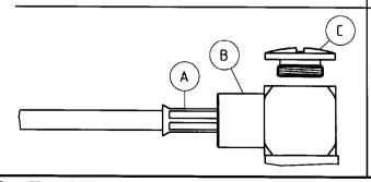
Slide ferrule A over braid and crimp as close to connector body B as possible.
