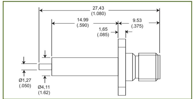
Straight Jack, Solder Pot Contact, Flush Dielectric
