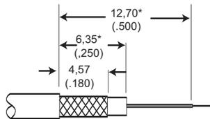
1. Trim cable to dimensions shown being careful not to nick or damage braids or center conductor. Trim center conductor. \* These dimensions suit 2,54 (.100) and 7,62 (.300) PCB pitches, for other pitches see Note 4.
