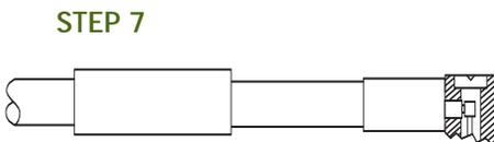
8. Slide heat shrinkable tubing over ferrule flush against body and heat until tubing shrinks down.
