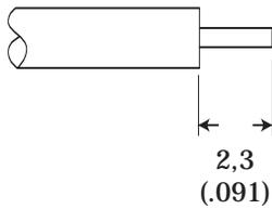
1. Remove the cable outer conductor and dielectric to the dimension shown taking care not to nick the center conductor using cable cutting tool. Deburr outer conductor at point of cut.
