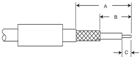
1. Trim cable to dimensions shown taking care not to nick braid or center conductor. Tin center conductor (DO NOT OVER TIN) then slip crimp ferrule over cable.
