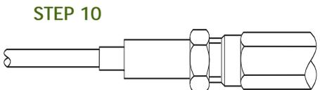
1. Slide ferrule and heat shrinkable tubing on to cable.
