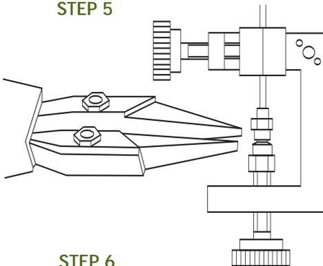
5. Place connector assembly in Assembly Jig T1848, or other suitable clamping arrangement, with contact in locator tool as shown.
