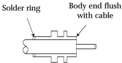
3. Clean housing area of outer conductor with abrasive paper and clean in a suitable agent. Ensure body is correct way round. Solder body ensuring end of cable to be flush with end of connector body as shown.
