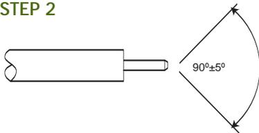
2. Point the end of the center conductor using a miniature file.
