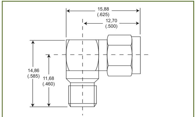
The surface finish on these products is passivated stainless steel. For gold plated versions change last three digits of the the part number from 890 to 310.
