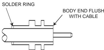
4. Clean housing area of outer conductor with abrasive paper and clean in a suitable agent. Place 24 s.w.g. soldering ring and connector body on prepared end of cable. Ensure body is correct way round. End of cable to be flush with end of connector body as shown.
