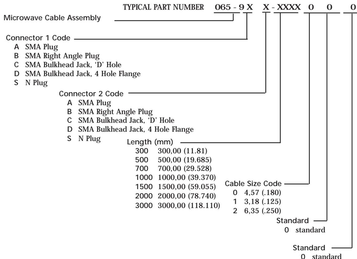
Example: 065-9AS-1000000 = Sealflex 2 cable assembly; 4,57 (.180) with 1 SMA plug and 1 N plug on 1 metre length of cable
