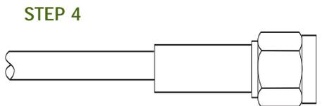
4. Slide ferrule flush against the body and crimp in position using Cannon's Crimp Tool and suitable Die Set (see table).
