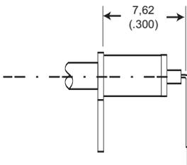
4. Bend center conductor to dimension shown depending upon preferred orientation. These dimensions suit 2,54 (.100) and 7,62 (.300) PCB pitches. For other pitches of 2,54 (.100) multiples add 2,54 (.100) multiples to the 12,70 (.500) and 6,35 (.250) dimensions in the cable stripping instructions Note 1.
