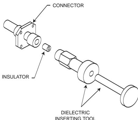
6. Using dielectric insertion Tool T2508 (for plugs) or T2509 (for jacks), press insulator into body. Assembly is now ready for use.
