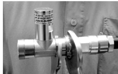
Coupling nut torque forces must not exceed IEC standard or manufacturer detail specifications (IEC: DIN 7/16 - 30 Nm max. and N - 1.13 Nm max.).
