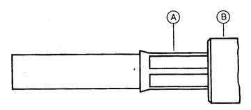
Slide ferrule A over braid and crimp as close to connector body B as possible. (Crimp insert: B, C or D).
