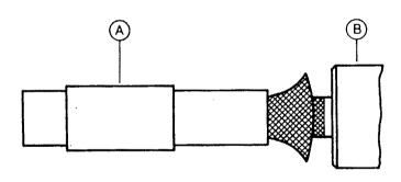
Splay out braid, and insert cable in connector body B. Ensure that braid lies above the crimp neck.
