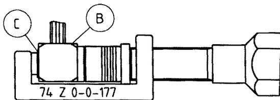
Locate cover C into rear opening of body B.
