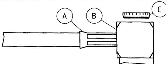
Slide ferrule A over braid and crimp as close to connector body B as possible
