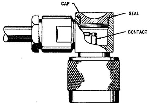
6. For access type angle connectors, solder center conductor in contact groove. Close access opening.
