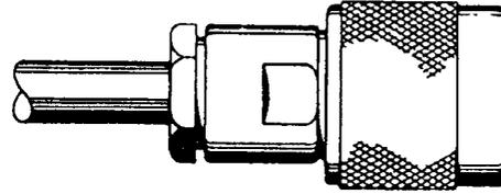
5. Thread assembly into connector, and lock securely. Vee gasket must be split by braid clamp.
