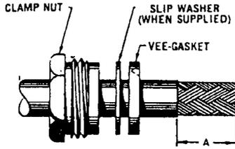
1. Cut cable end square, place clamp-nut, slip washer (when supplied), and gasket over jacket. Remove jacket to dimension "A."
