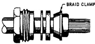
2. Comb out braid and taper forward. Place braid clamp over braid against jacket cut.
