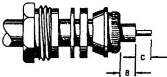
3. Fold braid back over braid clamp and trim as shown above. Remove dielectric to dimension "B." Cut center conductor to dimension "C."
