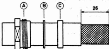
Slide nut A, washer B and gasket C over cable. Remove carefully 26 mm of cable jacket without damaging or opening the braid.
