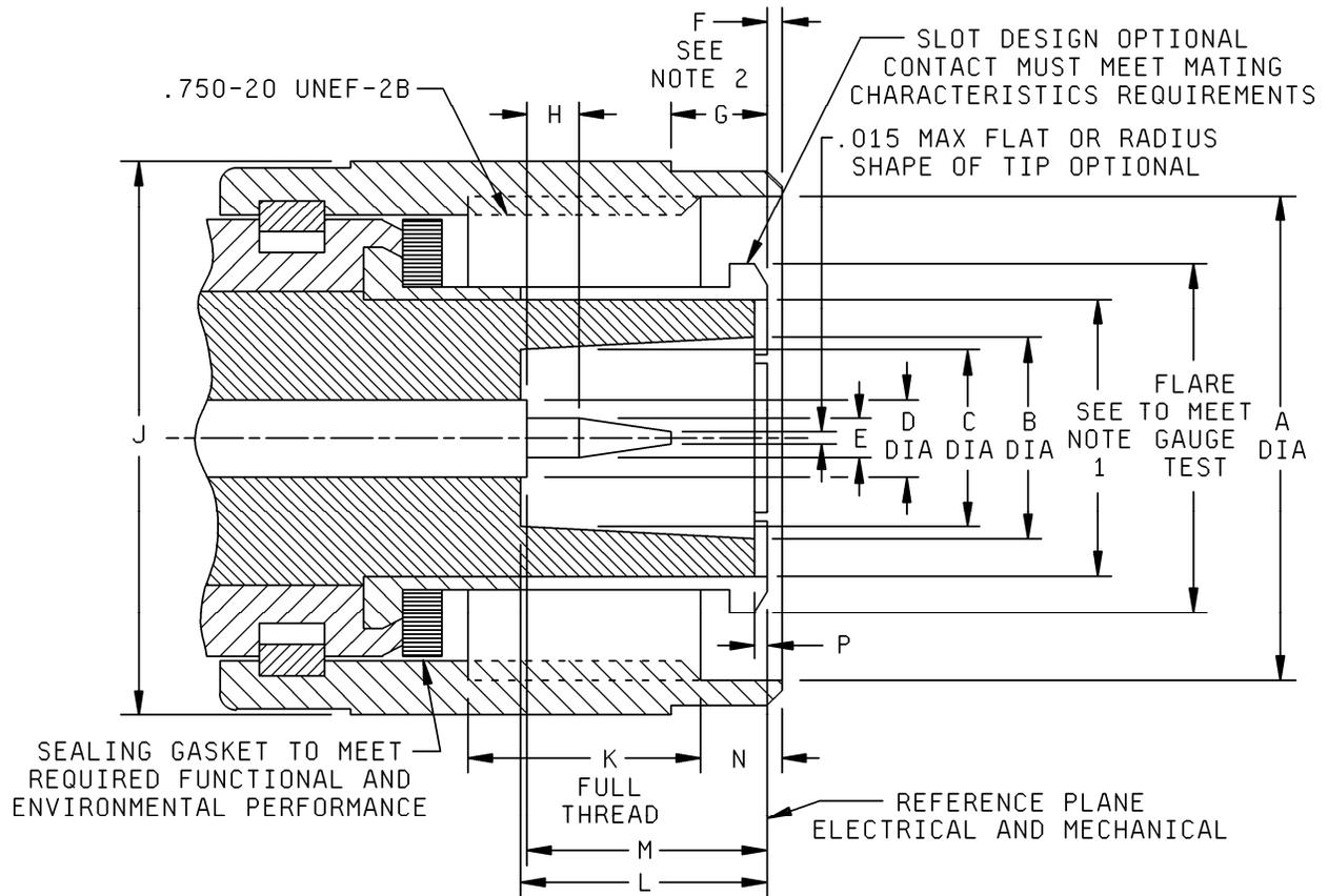
FIGURE 57. Interface, series HN, pin contact.
