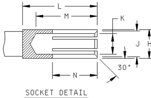
FIGURE 50. Interface, series LC, socket contact
