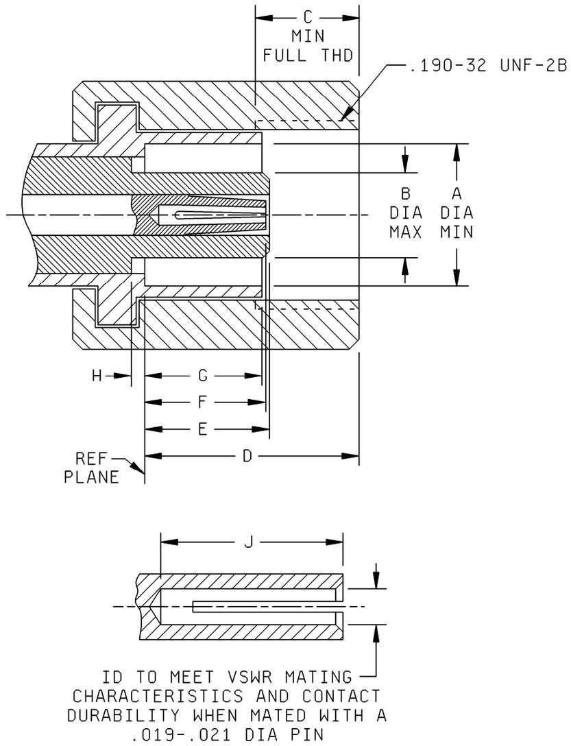
FIGURE 40. Interface, series SMC, socket contact.
