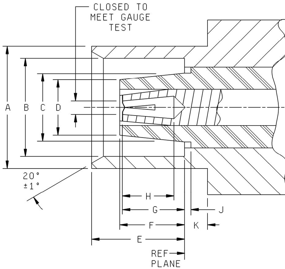
FIGURE 72. Interface, series BMZ, socket contact.
