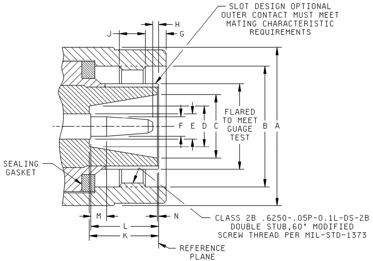
FIGURE 30. Interface, series QSC, pin contact.
