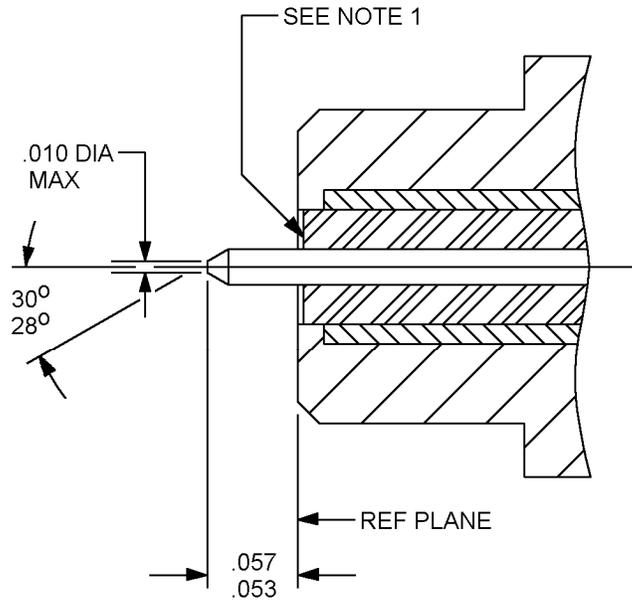
THE CABLE CENTER CONDUCTOR IS USED AS THE CENTER CONTACT PIN
