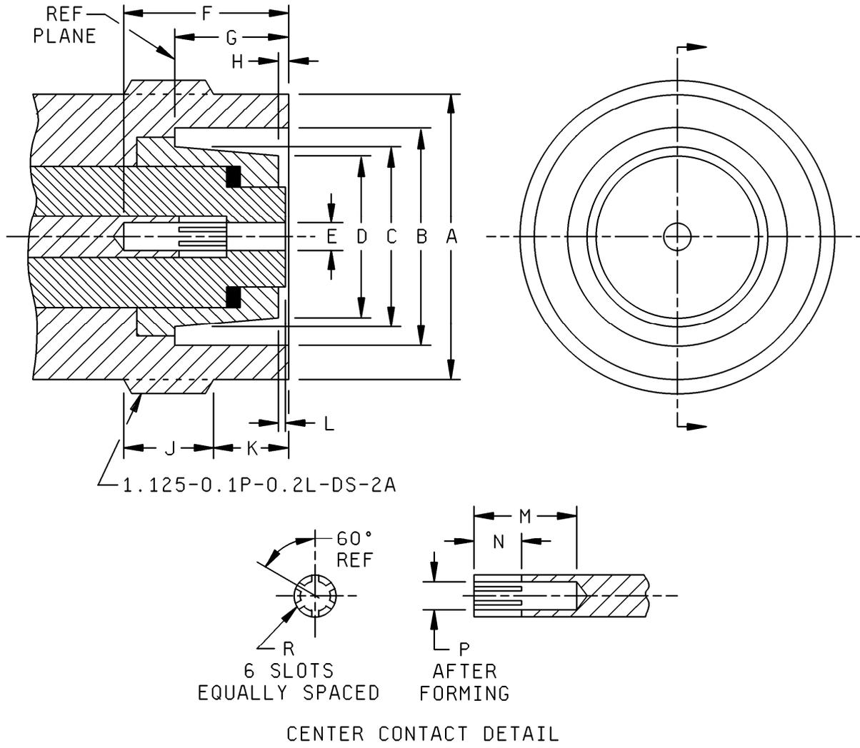
FIGURE 27. Interface, series QM, socket contact.
