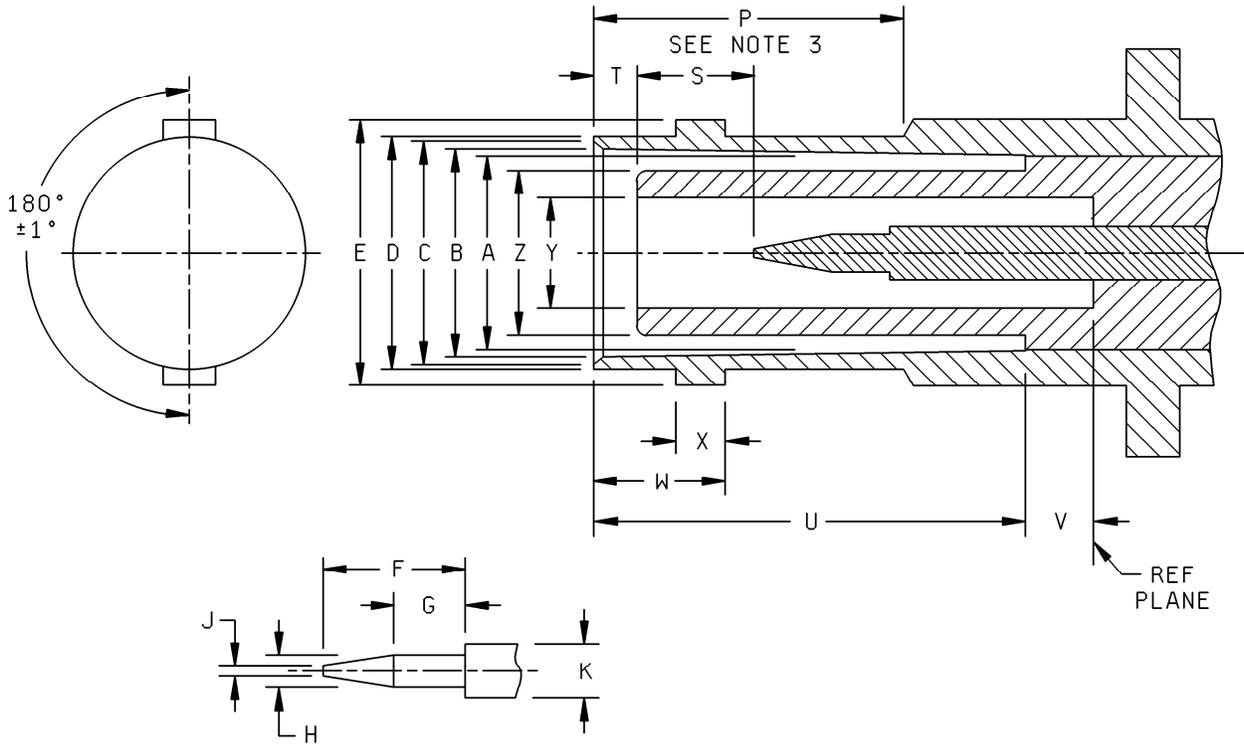
FIGURE 45. Interface, series SHV, pin contact.
