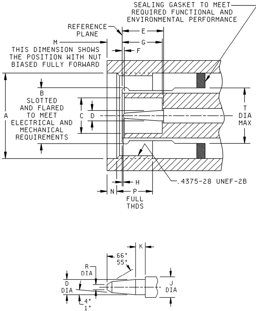
FIGURE 41. Interface, series TNC, pin contact.
