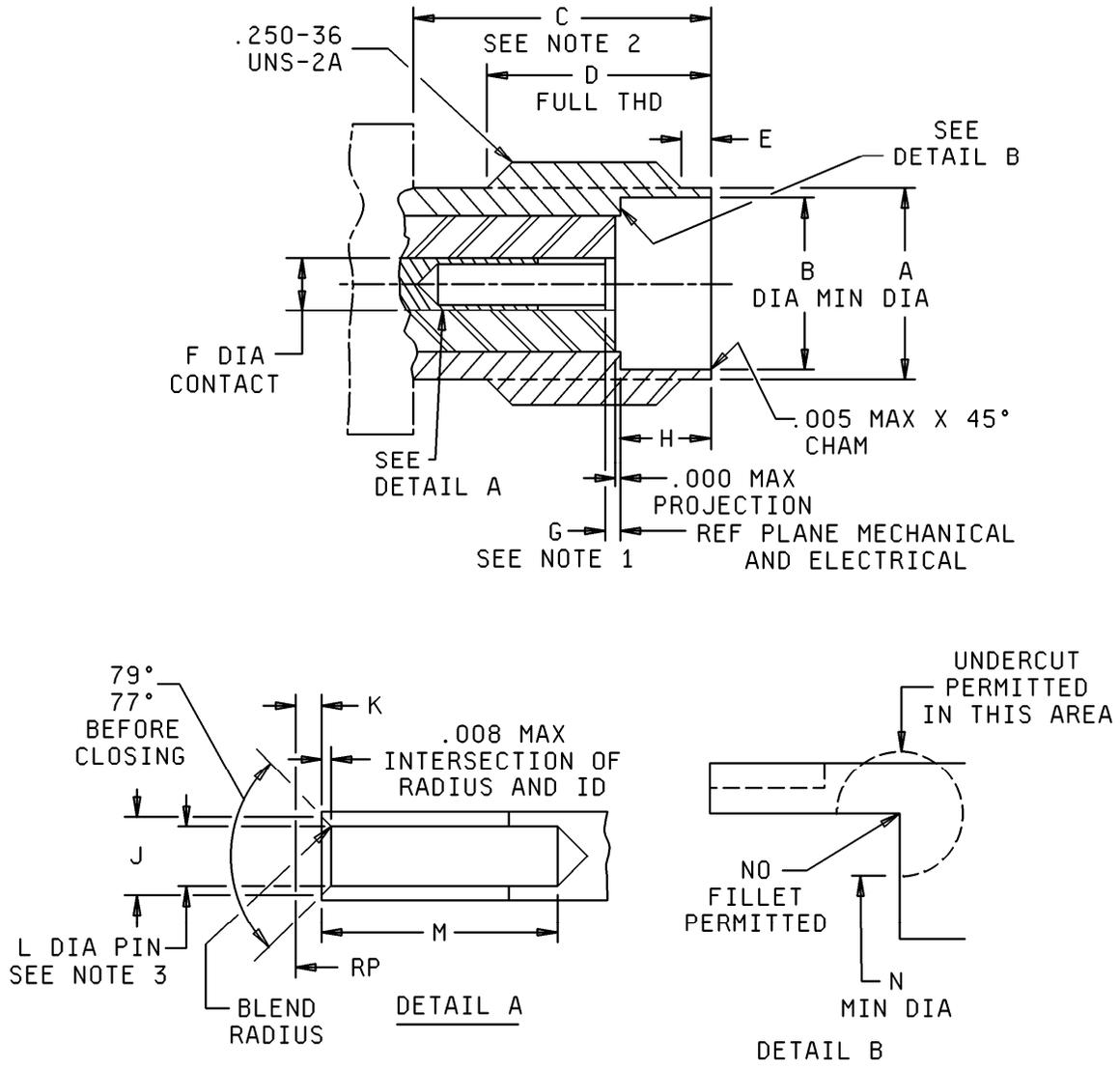
FIGURE 35. Interface, series SMA, socket contact.
