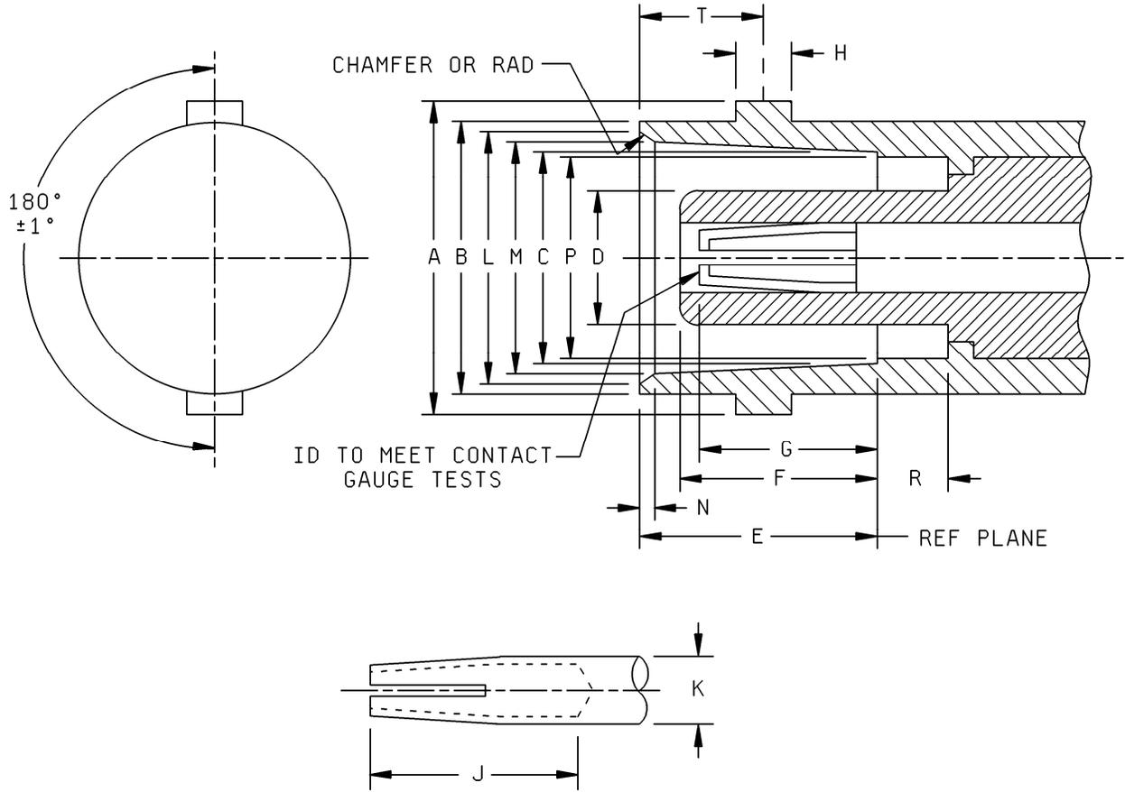
FIGURE 21. Interface, series MHV, socket contact.
