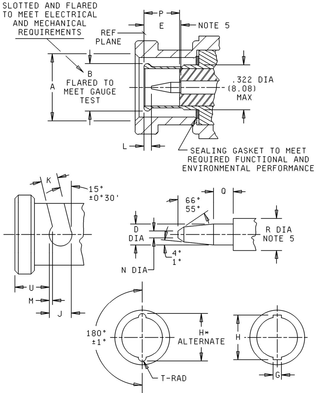
FIGURE 85. Interface, series BNC, pin contact, 75 ohm.
