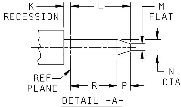
FIGURE 67. Interface, series BMB, pin contact.
