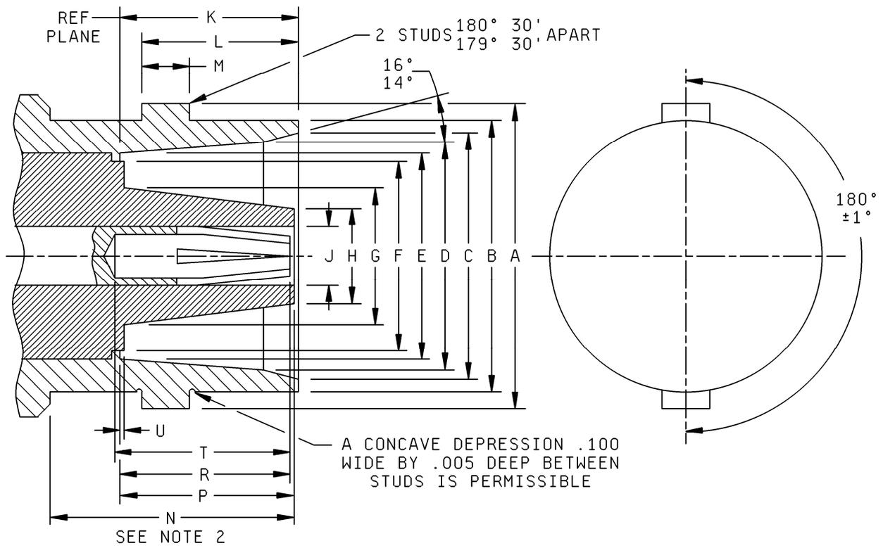
FIGURE 19. Interface, series C, socket contact.
