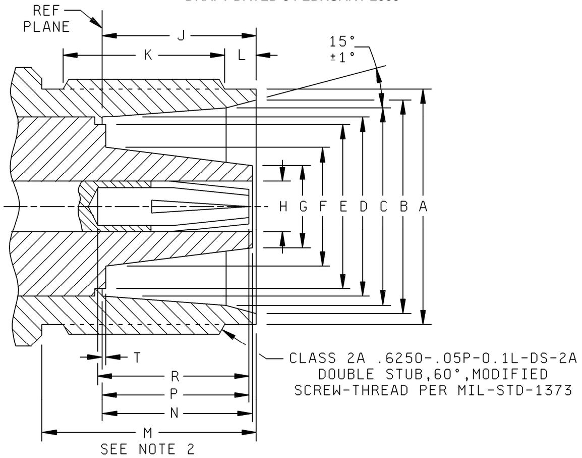
FIGURE 31. Interface, series QSC, socket contact.
