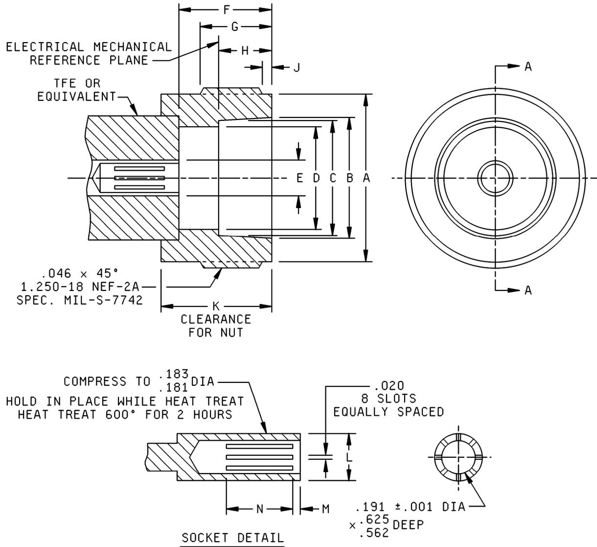
FIGURE 60. Interface, series LT, socket contact.
