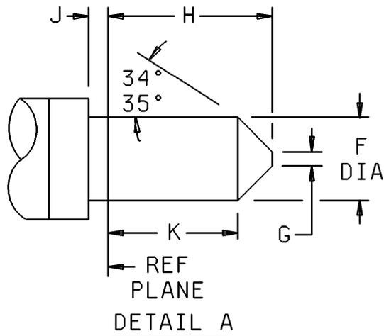
FIGURE 34. Interface, series SMA, pin contact.
