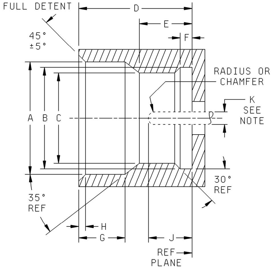
FIGURE 75. Interface, series SMP, pin contact, full detent.
