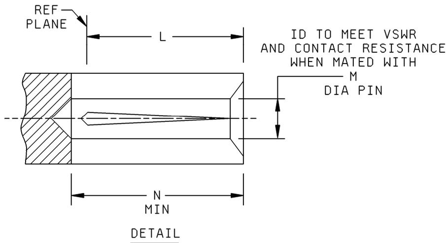
FIGURE 23. Interface, series N, socket contact.
