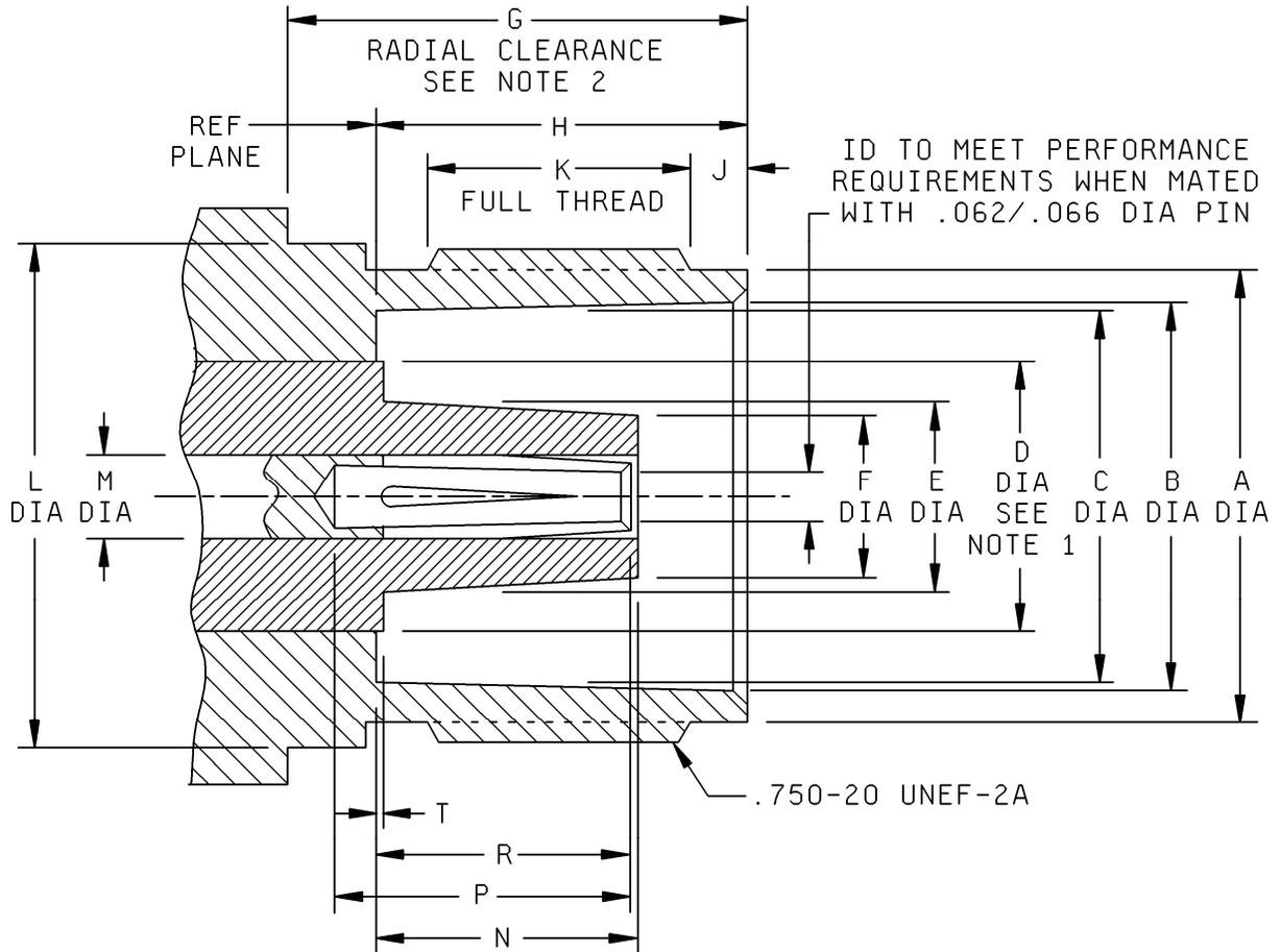
FIGURE 58. Interface, series HN, socket contact.
