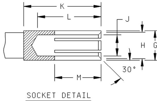
FIGURE 48. Interface, series LC, socket contact, full dielectric.
