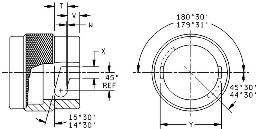
FIGURE 18. Interface, series C, pin contact.
