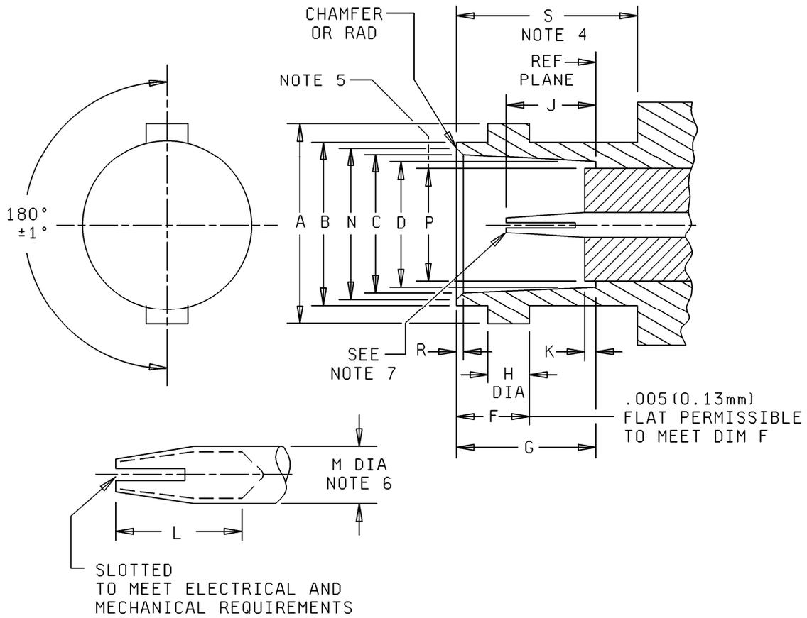
FIGURE 84. Interface, series BNC, socket contact, 75 ohm.
