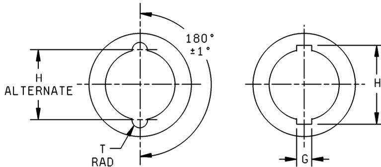
FIGURE 16. Interface, series BNC, pin contact.
