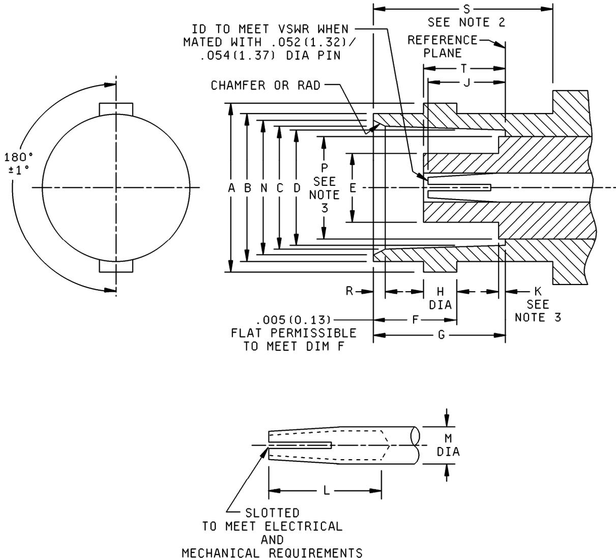
FIGURE 17. Interface, series BNC, socket contact.
