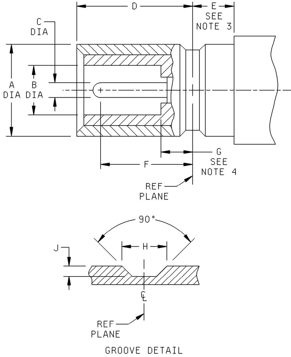
FIGURE 63. Interface, series SSMB, pin contact.
