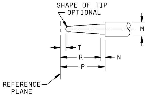
FIGURE 28. Interface, series QNC, pin contact.
