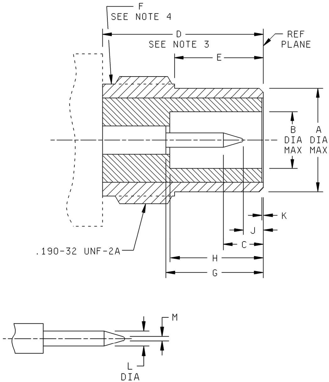
FIGURE 39. Interface, series SMC, pin contact.
