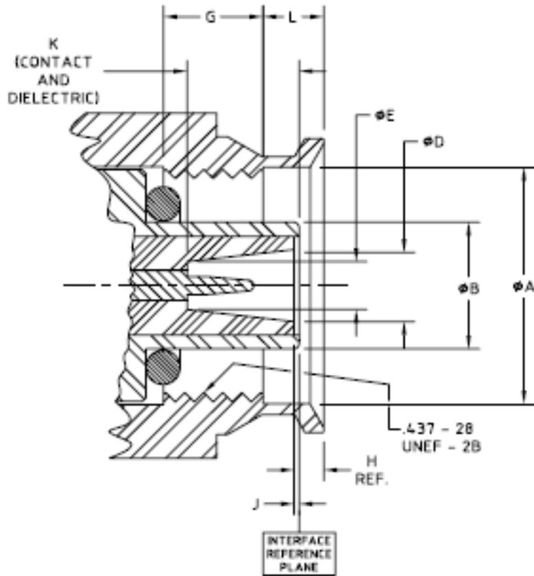
FIGURE 83. Interface, series TK, pin contact, unslotted outer contact.
