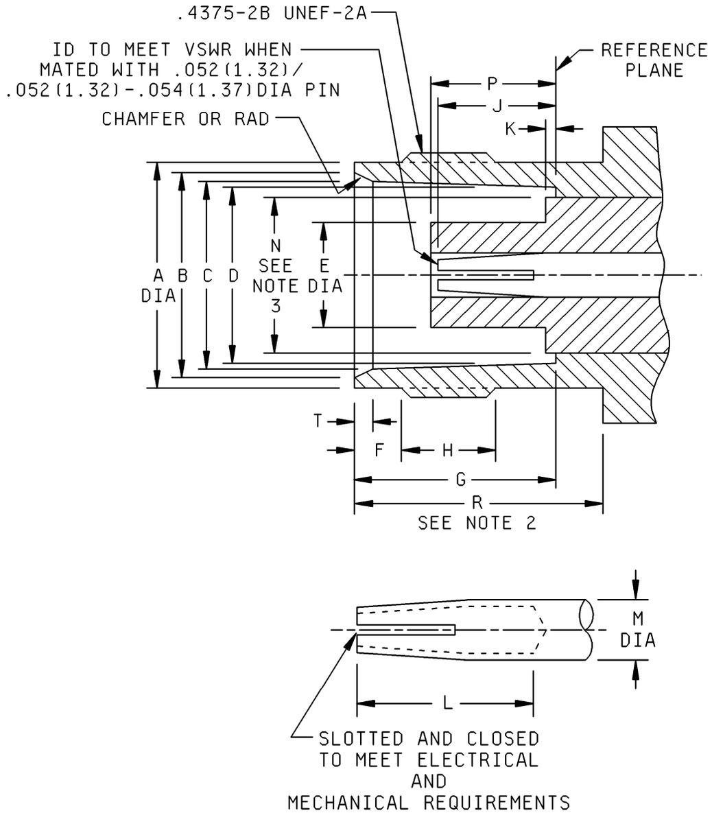
FIGURE 42. Interface, series TNC, socket contact.
