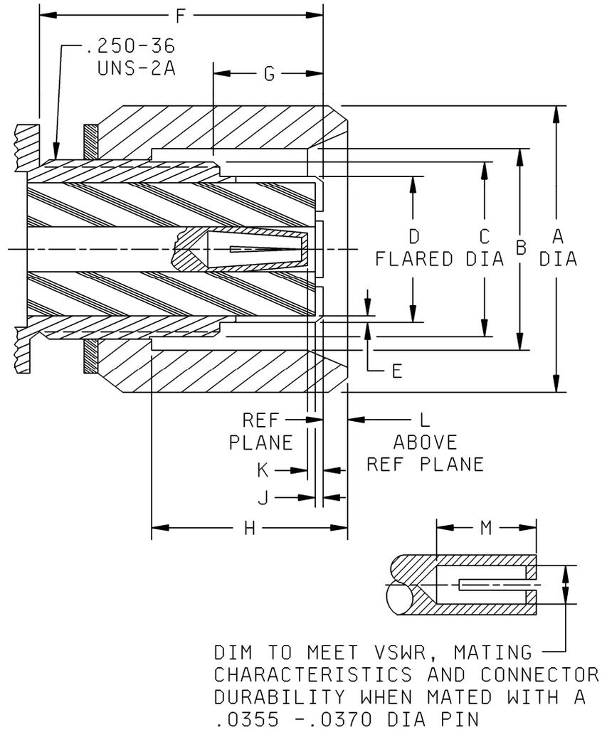
FIGURE 68. Interface, series BMB, socket contact.
