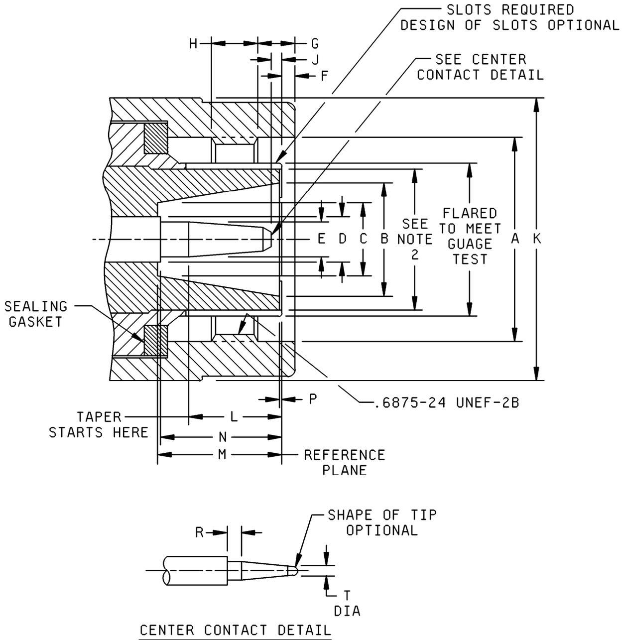
FIGURE 32. Interface, series SC, pin contact.
