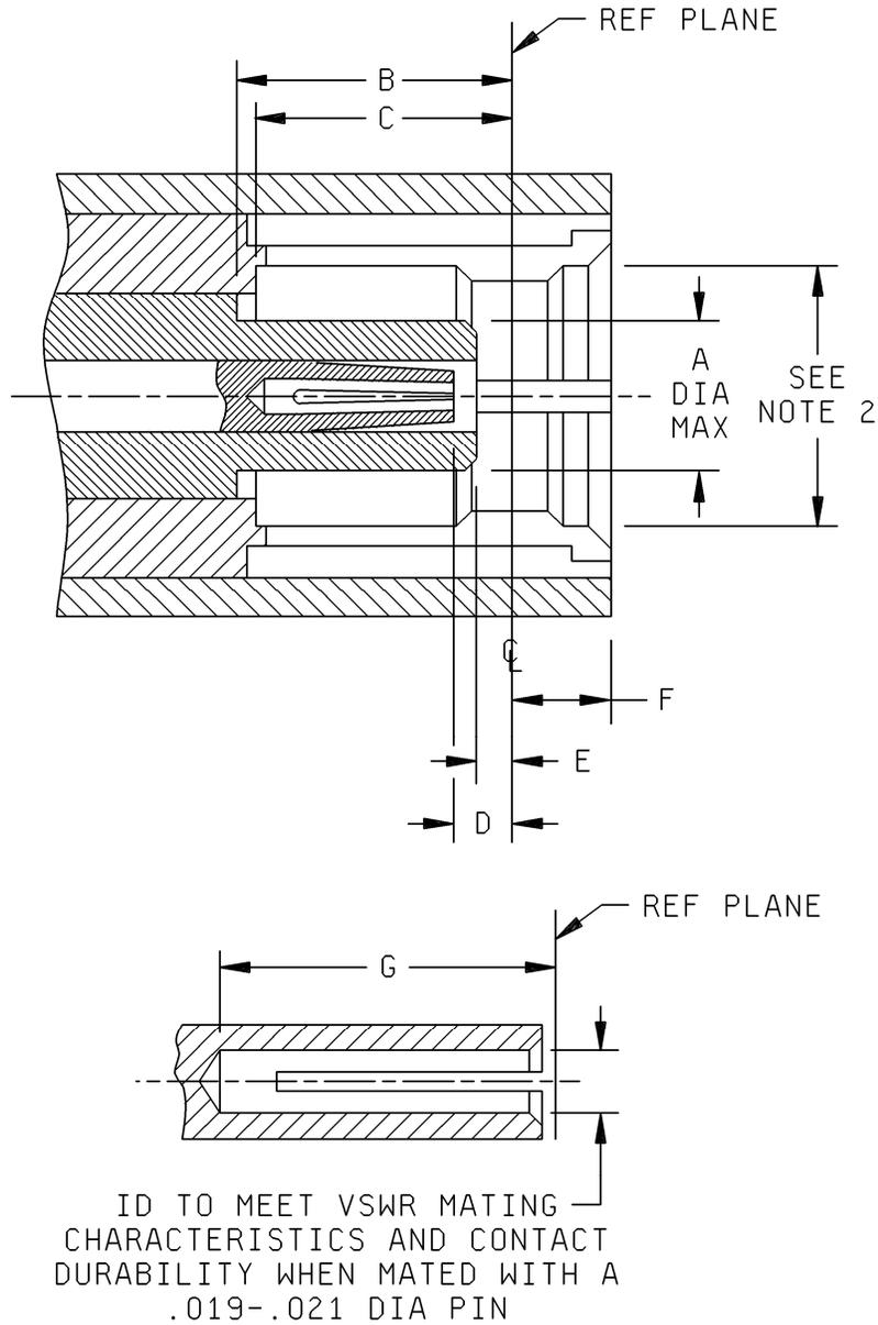
FIGURE 38. Interface, series SMB, socket contact.
