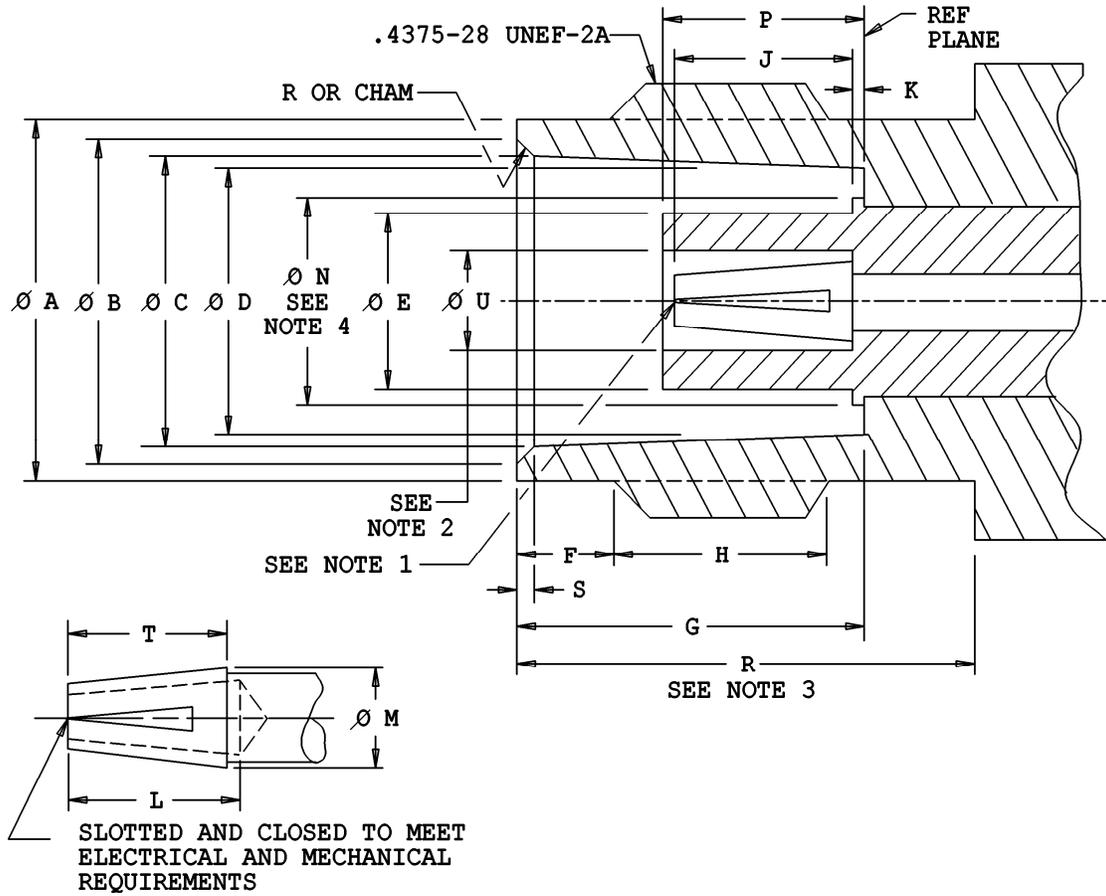
FIGURE 44. Interface, series TNCA, socket contact, air interface.
