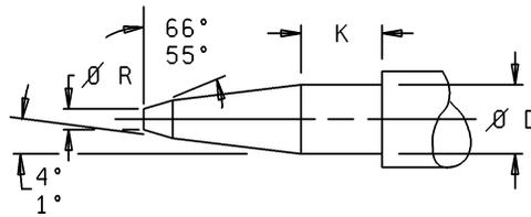
FIGURE 43. Interface, series TNCA, pin contact, air interface.
