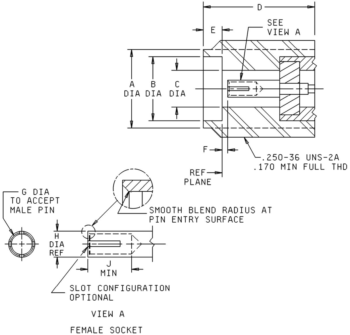
FIGURE 70. Interface, series SMK, socket contact.
