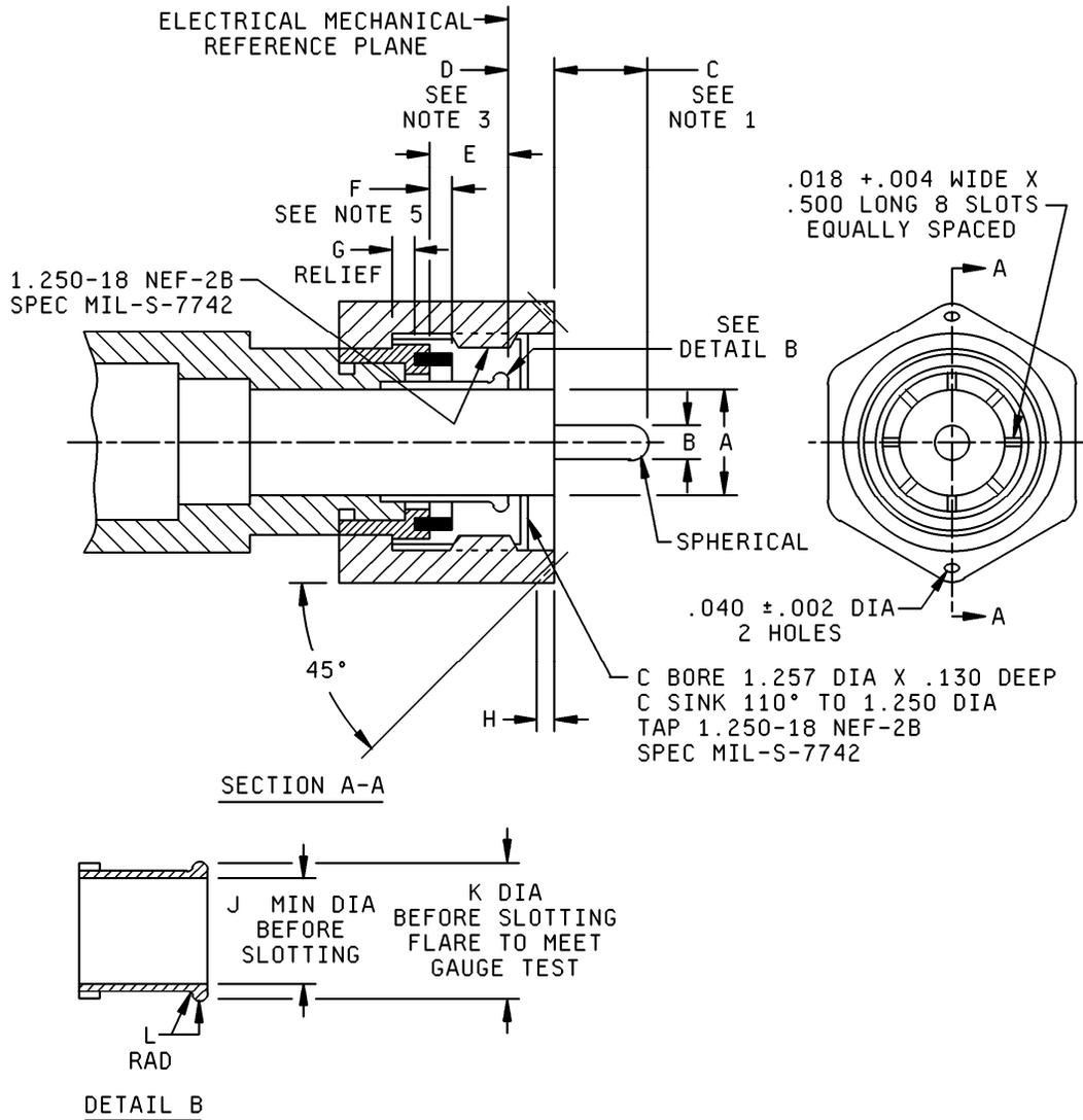
FIGURE 59. Interface, series LT, without contact.
