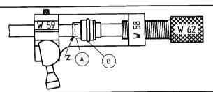
IMPORTANT: Remove O-Ring gasket C from connector housing A prior to soldering. Slide connector housing A onto cable. Place cable in soldering fixture W 58 and fix between inserts W 59. Tighten locator tool W 62 completely against cable end. Push connector housing A completely against locator tool W 62. Solder connector housing A to cable by z, avois excessive heat, immediately cool down and clean with alcohol.
