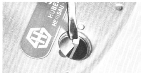
Remove cover-screw. Release spring catch with screwdriver. Replace screw. (This interference is subsequently detectable owing to the red colour seal).
