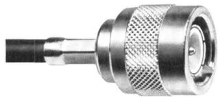
Precision coaxial connector, bayonet coupling mechanism, corrosion-resistant, for cable sheath diameters 4.9–11.4 mm.
