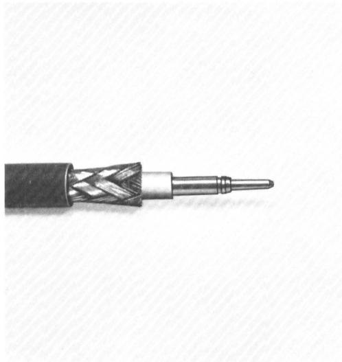
Push dielectric into cylindrical insert of the small recess of the crimp die.
