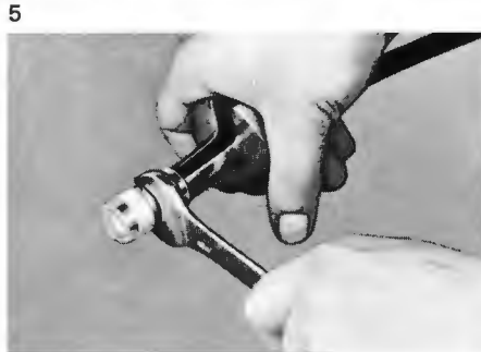
Assembly of FUK Cable-Entry Construction
