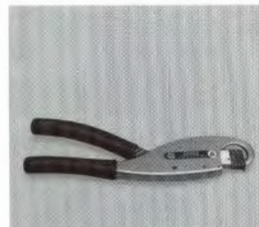
Small crimp tool with fixed insert
