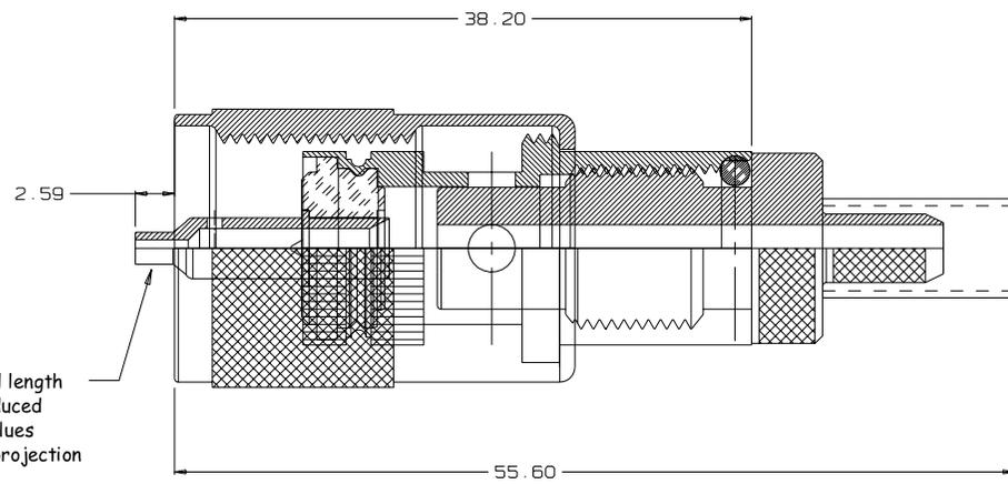
The contact overall length may need to be reduced to match typical values between 1~1.5mm projection
