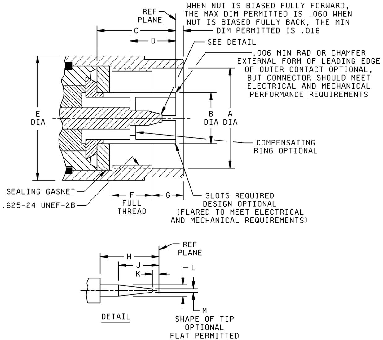
FIGURE 22. Interface, series N, pin contact.
