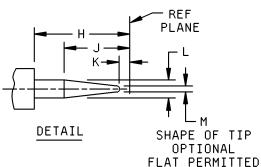
FIGURE 22. Interface, series N, pin contact.
