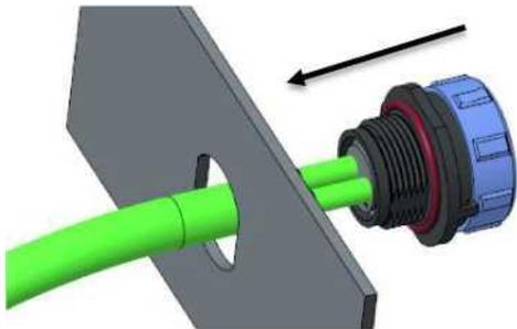
4.Tighten the retaining nut according to the torque.
