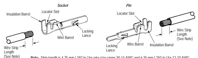
Note: Strip length is 4.75 mm [.197 in.] for wire size range 30-14 AWG and 6.35 mm [.250 in.] for 12-10 AWG.
