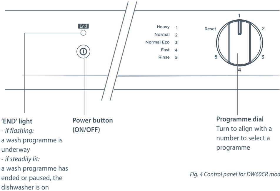
Fig. 4 Control panel for DW60CR models
