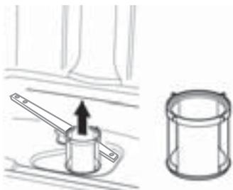
Fig. 12 Removing the filter unit (Filter B)
