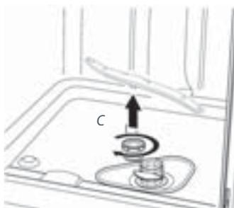
Fig. 13 Removing the spray arms (C and D)
