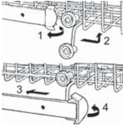
Fig. 6 Adjusting the upper rack for DW60CR models
