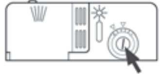
Fig. 9 Adjusting the dose regulator
