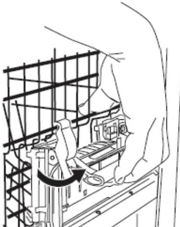
Fig. 7 Adjusting the upper rack for DW60CD models
