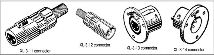
Cannon rearranged the pins and added a latch, and the XL (X series with Latch) was born. One of the great features of this connector is that the female pin 1 contact was placed forward in the shell and thus made connection first and broke connection last. Since pin 1 was used for the cable shield this greatly reduced the chance for hum or buzz as connectors were plugged and unplugged. This is the connector others such as Switchcraft and later Neutrik have copied.
