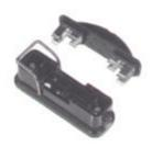
A strong fusebox which has been designed to take 32mm x 6.3mm fuse links which are held in the lid and automatically exposed and isolated from the circuit when the lid is raised. Leads may be inserted through the base or through the ends of the box. The lid is retained by a spring.
