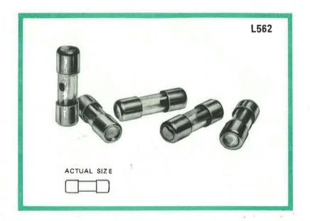
These fuse links have a minimum life of 1,000 hours at rated current, at  $20^{\circ}$ C The higher ratings (250 mA and over) blow within 10 seconds at twice their rated current, lower ratings at  $3 \times Ir$ .
