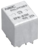
The NEC TOKIN EP1K Series are PC-board mount automotive relay suitable for control of heaters, fans and pumps, etc. The EP1K relay was developed based on the EP1 relay, and the performance of carrying current is about 10A larger than the EP1 relay.
