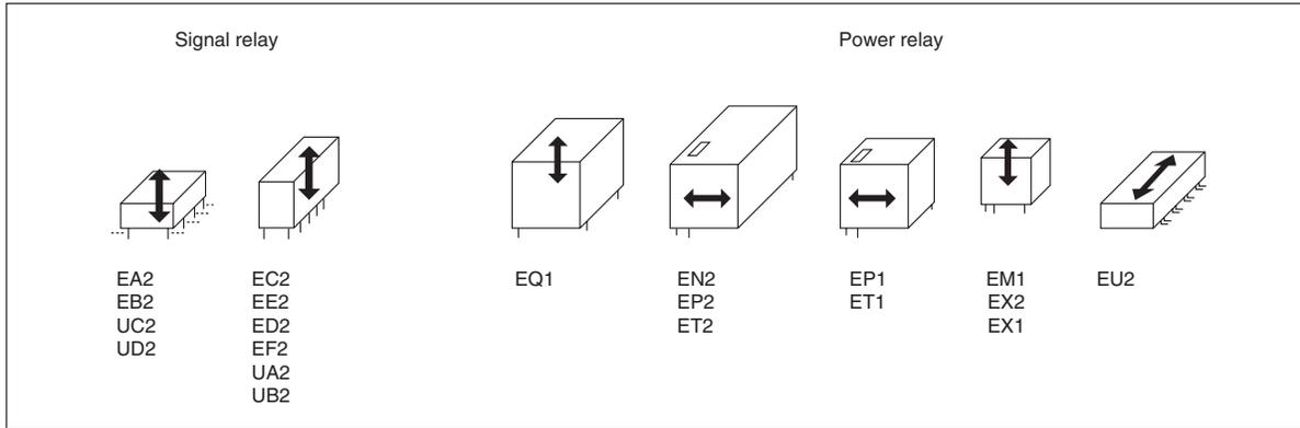
Fig.10 Direction of Armature Operation
