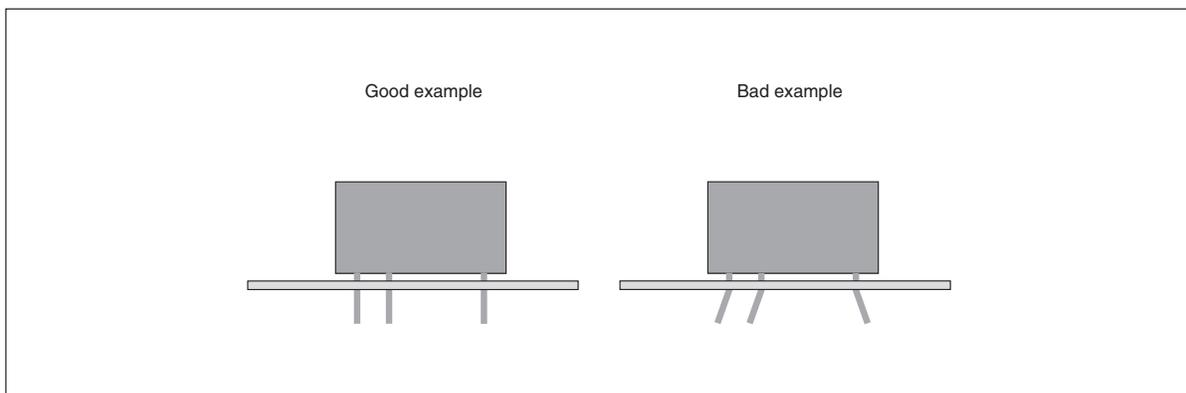
Fig.11 Bending Relay Pins
