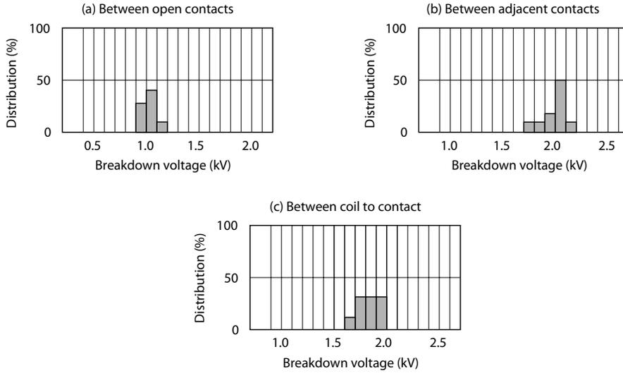
ALTERNATION OF VOLTAGE AT DENSELY MOUNTING (Magnet interference)
