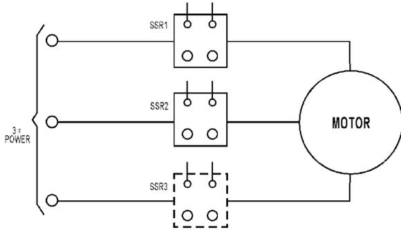
Three-phase motors may be controlled by solid-state relays as shown. A third SSR as shown is optional, but not necessary. The control windings may be connected in series or parallel. Care should be taken to ensure that the surge current drawn by the motor does not exceed the surge current rating of the SSR.
