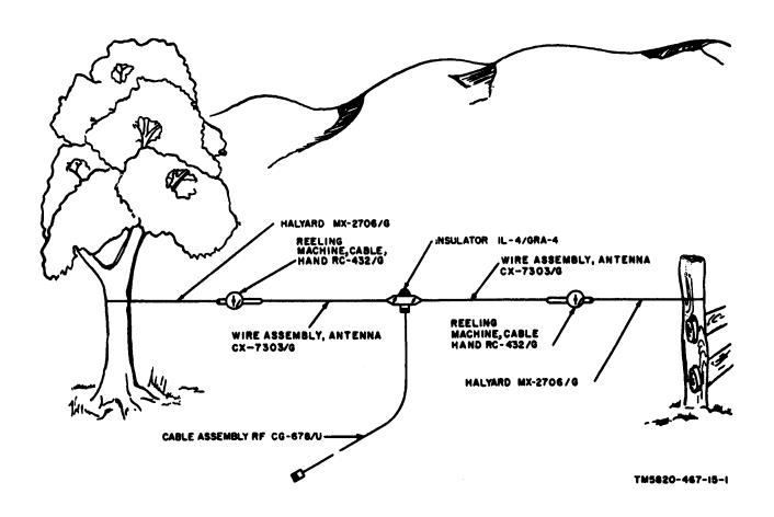
Figure 1. Antenna Group AN/GRA-50, typical installation.
