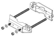
for use with most 1-point mount Cellular panel antennas Mast dia. 2-4.5 inches (50-115 mm) Weight 2 lb (0.9 kg)
