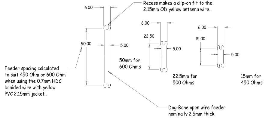
Material is 2~2.5mm thick low-loss UV stable plastic semi-rigid sheet (clear or colour of choice) with tolerance for clip-on tension as required to grip on the yellow PVC insulaton of the Antenna Wire (CASA FS Specification).
