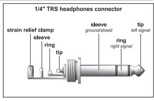
Fig. 3.4: Stereo plug for headphones connection
