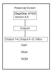
Figure 2.18. Output parameters LCD submenu
