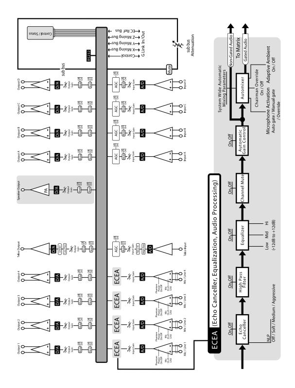
Figure F.3. Audio flow block diagram
