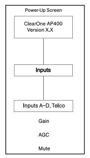
Figure 2.16. Inputs A-D submenu
