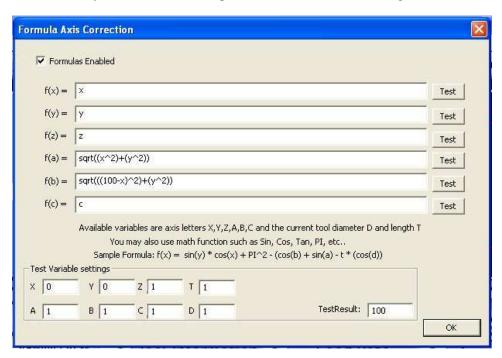
Here the equations have been entered into the dialogue box and the enable formulas box checked. With x = 0 and y = 0 in the variable test settings I get zero when I click test for A and 100 when I press test for B. This is because d was set to 100.
