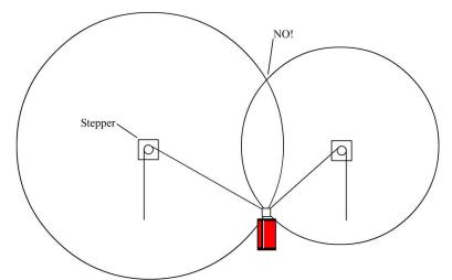
Hektor's struts" force" the spray can to lie on the intersection of two circles but gravity chooses the lower intersection.
