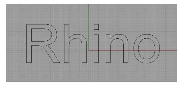
Select the lines and type divide in the command line and accept the seam adjustment. Type L and press return to allow the segment length to be defined and then enter the segment length you want.
