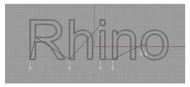
The drawing is now covered in dots that are the distance apart you specified. We will use these to split the drawing into little segments. Type split and when asked for the cutting object select all of the points by dragging a box or type SelPt and press return. Then press return and the lines will be split up
