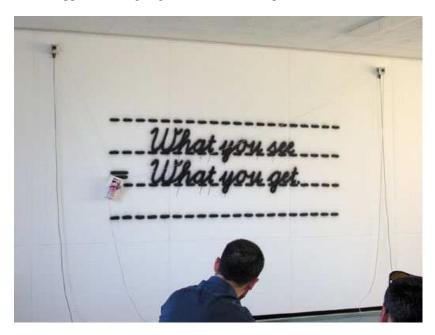
This is Hektor in action, see <a href="http://www.hektor.ch">http://www.hektor.ch</a> for more details and art. The system works by hanging a solenoid operated spray can by two toothed belts that can be fed in and out by steppers. Gravity sorts everything else out.
