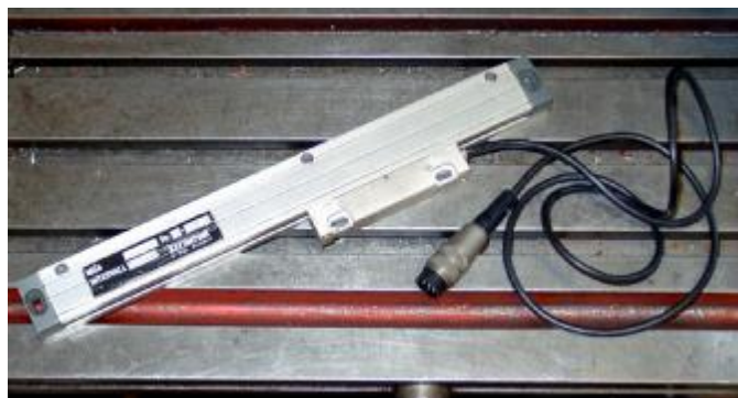
Figure 4.16 - Glass scale encoder (awaiting installation)
