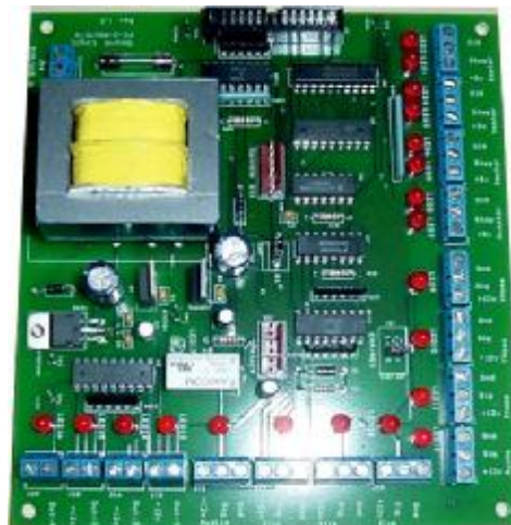
Figure 4.2 – Two examples of commercially available breakout boards
