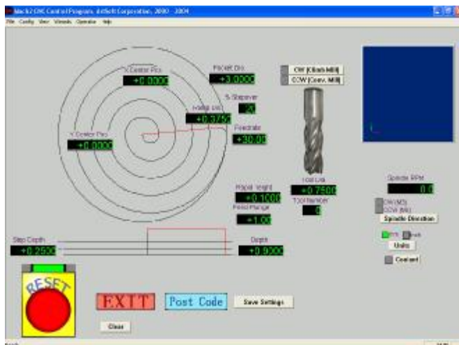
Figure 3.8 – Circular pocket with defaults
