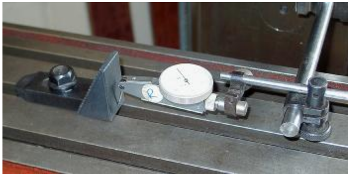
Figure 5.12 - Establishing a zero position
