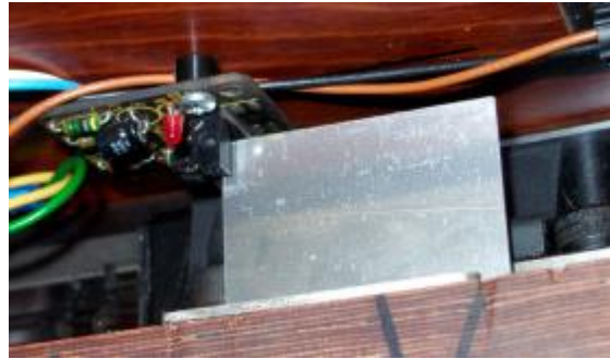
Figure 4.8 - Optical switch on table with vane on bed of machine
