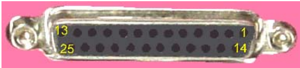
PulsePacer Output Plug Pin Numbers
