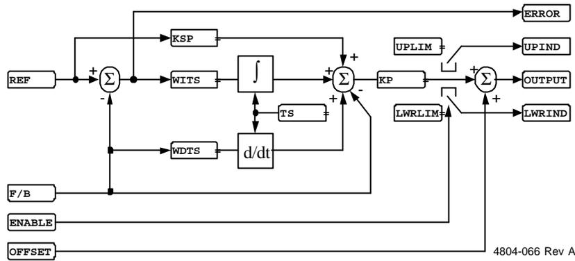
Figure 4.3: PID Controller special function module
