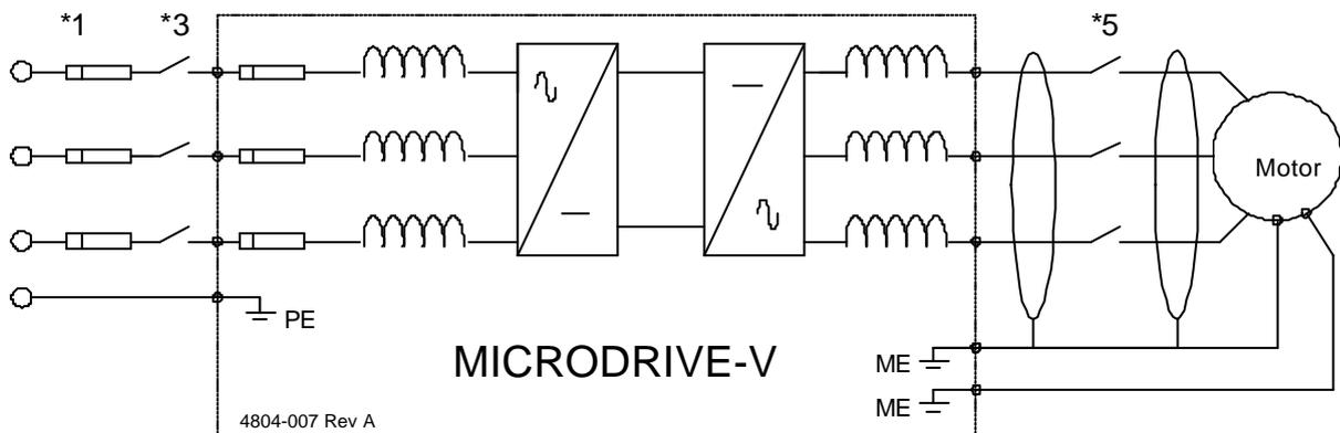
Figure 3.1: Power Connection Details
