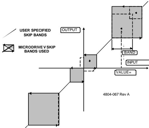
Figure 4.4: Skip bands special function module
