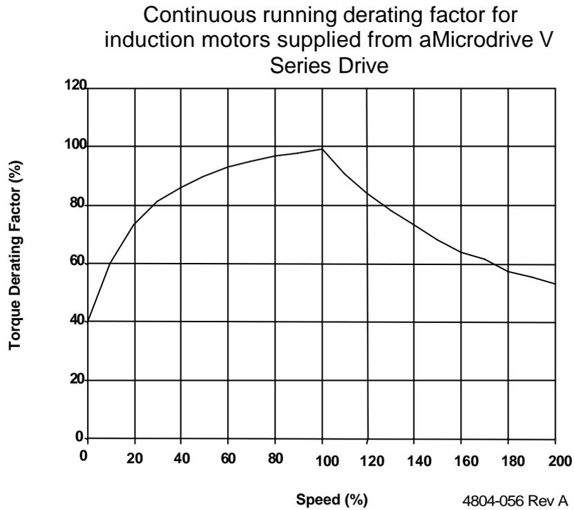
Figure 2.8: Microdrive V Series Typical Motor Derating Curve
