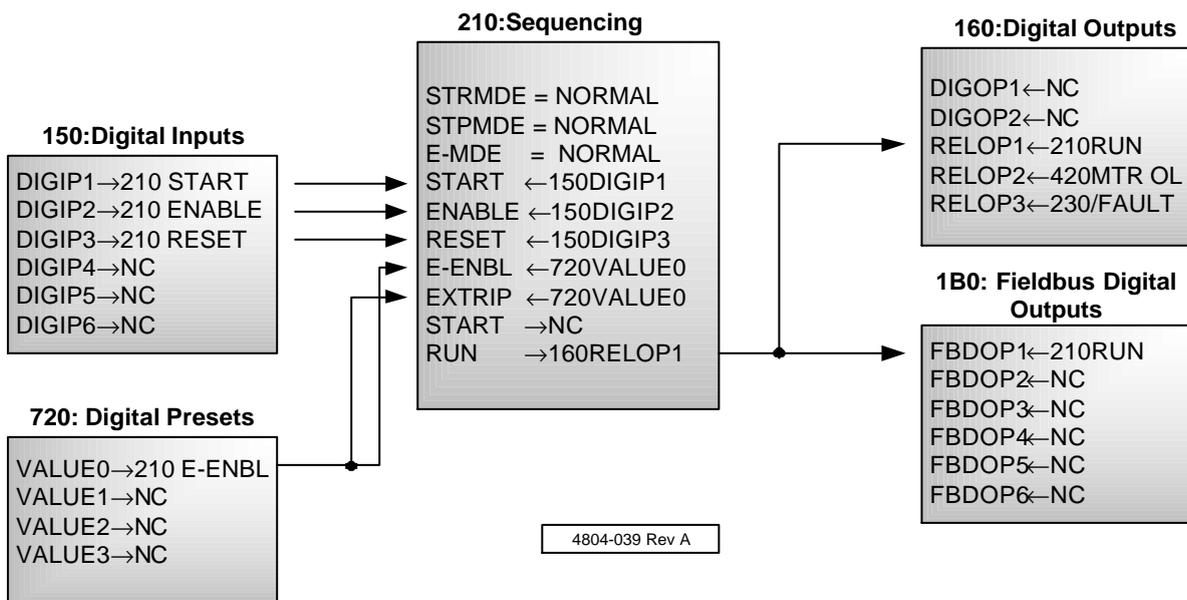
Figure 2.5: Example configuration for simple speed control (part of the default setup)
