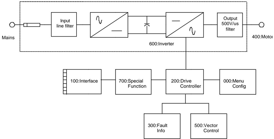
Figure 2.3: Microdrive V Series Block Diagram
