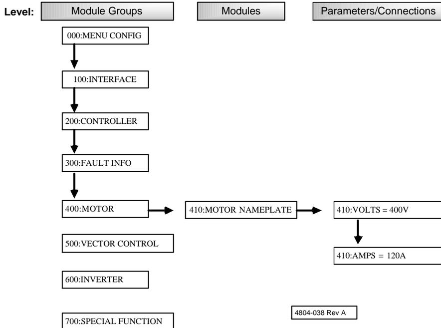
Figure 2.4: Menu navigation example - setting motor nameplate current
