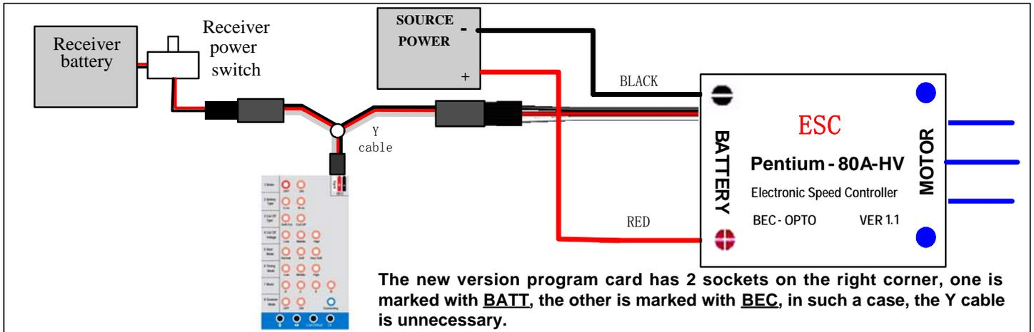
When you are using a program card to program the Pentium series HV ESC, the "Music/Li-Po cell" item now means the lithium battery cells number. (● = LED is lighting)
