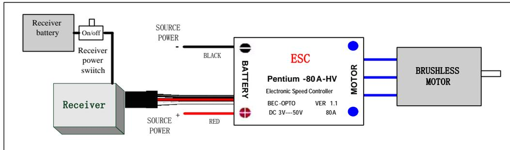
**Note:** For HV controller, the processor gets its power supply from the receiver, so if you want to restart the HV controller, you should take the control wires out of the receiver and then plug the wires into the receiver again. The reconnection of main source power cannot restart the HV controller.
