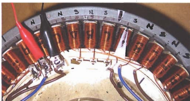
Fig.1: the first steps from Table 1 starting from zero at A+, B-. Note that the relevant polarity can be seen from the position of the alligator clips. A positive voltage makes the relevant winding a south pole, for example A+, B- makes the A winding south and the B winding north.
