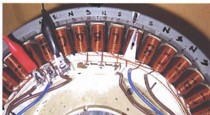
Fig.1: the first steps from Table 1 starting from zero at A+, B-. Note that the relevant polarity can be seen from the position of the alligator clips. A positive voltage makes the relevant winding a south pole, for example A+, B- makes the A winding south and the B winding north.
