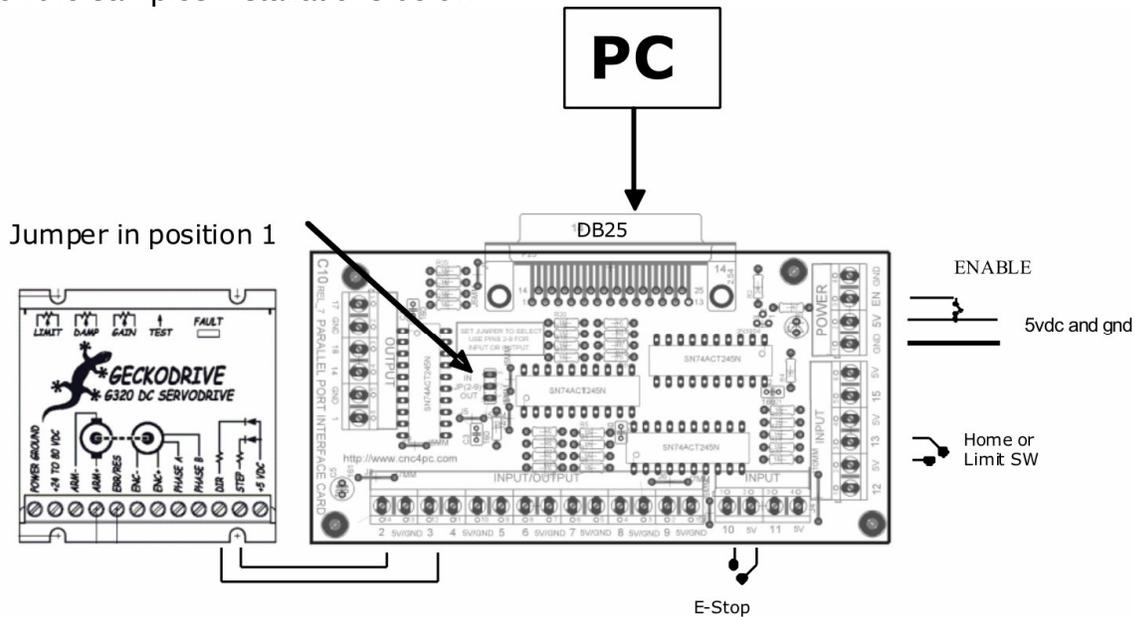
Sample wiring using pins 2-9 for output. Jumper must be in position 1.
