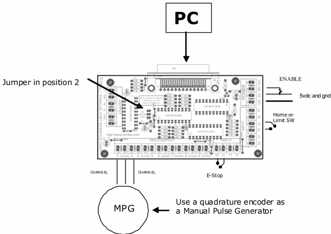
Sample wiring using pins 2-9 for input. Jumper must be in position 2.
