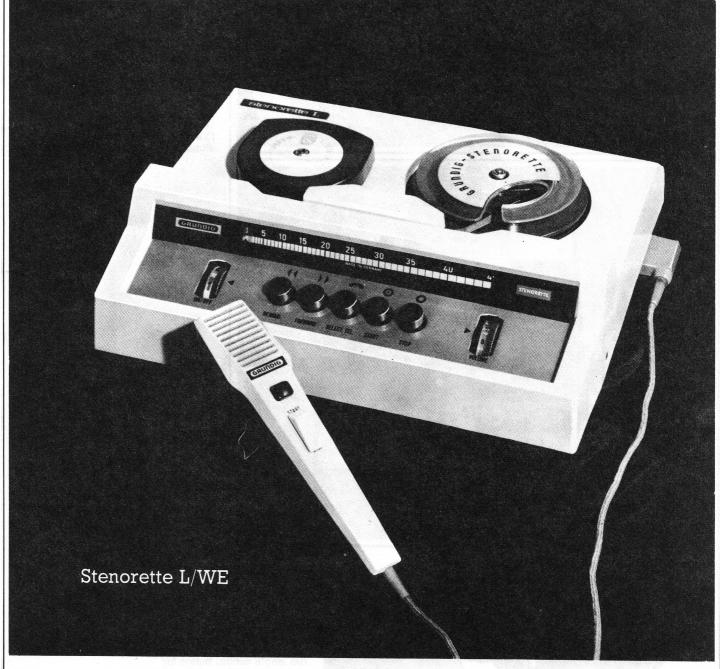
Executive-styled office dictation/ transcription machine with ensured split second accuracy for recording. Tape cassettes take 25 minutes recording, spools up to 45 minutes. Full remote facilities (start/stop/ backspace/record/playback) on the microphone. Adjustable sensitivity allows personal or conference recording.
