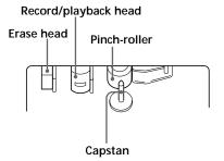
Wipe the heads, pinch roller and the capstan with a cotton swab moistened with alcohol every 10 hours of use.
