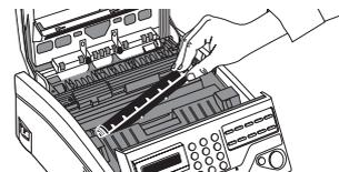
6. Once the toner cartridge is in place, push the coloured lever all the way forward to secure it and release the toner.
