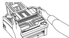
2. Grasp the control panel. Pull upward and toward you until it releases. Swing the control panel out of the way.
