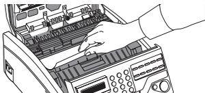
5. Place the image drum unit back into your fax machine. Ensure that the tabs on both sides of the image drum are inserted correctly as shown. Then press down firmly on both ends of the image drum until it snaps into place.
