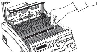
4. Remove the new toner cartridge from its package and gently shake it from side to side to distribute the toner. Then carefully peel the white plastic tape from the bottom of the toner cartridge.
