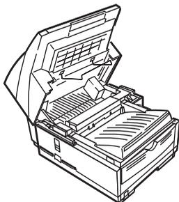
3. Press on the latches on both sides of the copier stacker until the cover of the image drum compartment is clearly released and pops up. Lift up and back, revealing the image drum unit.
