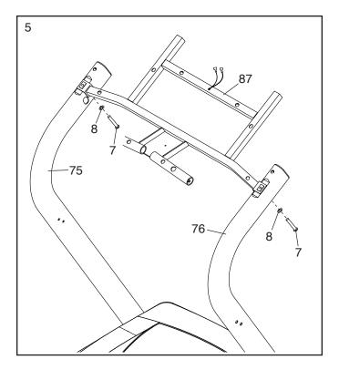
Insert the upper end of the Left Handrail (71) into the tube on the Console Frame (87). Hold the lower end against the Left Upright (75).
