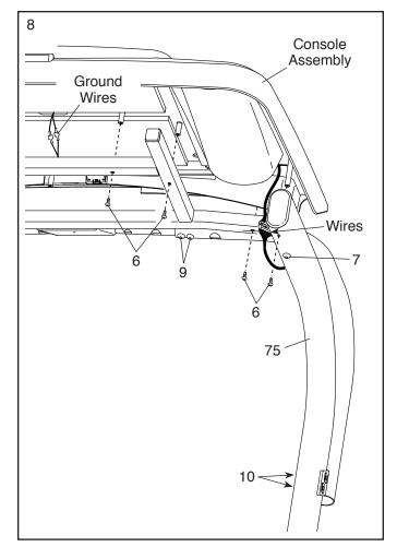
Attach the Pulse Bar Bottom (90) to the console assembly with six #8 x 3/4" Screws (6); start all six Screws, and then tighten them. Do not overtighten the Screws.
