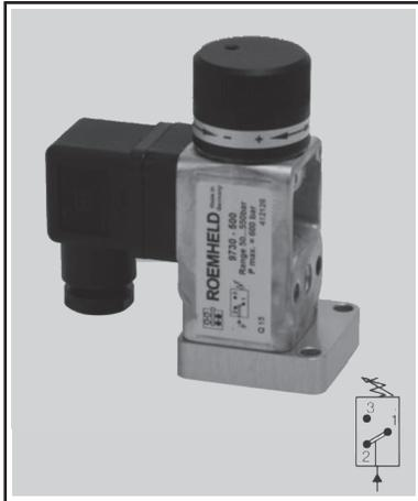
Hydra-electric pressure switches are devices which close or open electrical contacts under pressure. They are used to switch on or off pump motors, valves, machine tool interlocks or similar applications in power units, machines
