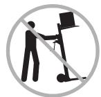
Do not move the machine with a raised load, except for minor positioning.
